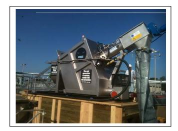
During the four-week test, the Beast processed 350,000 gallons of pure FOG. The majority of the FOG processed consisted of red cooking oil, humus, wet well lard and rags. No hot water, high pressure water or solvents were used and there was no rock trap or grinder. All trucks discharged directly into the Beast influent tank.
